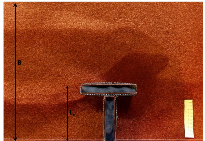
Figure 1. Geometric parameters of the spur dike
