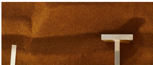
Figure 4. A view of the final scour profile in a T-shaped all-rigid spur dike
