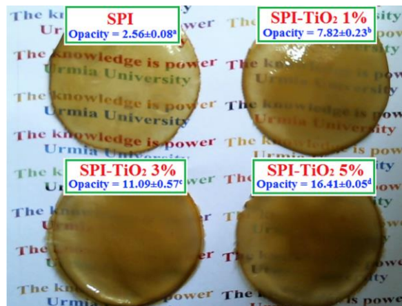
Figure 6. Appearance of the sesame protein isolate (SPI)- \text{TiO}_2 nanocomposite films and their calculated opacity values (Fathi et al., 2019).
